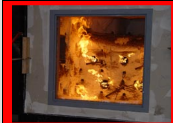
A Research-Scale Vertical Window Test at WFCi.
