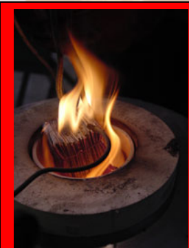
An ASTM D 1929 at WFCi.
