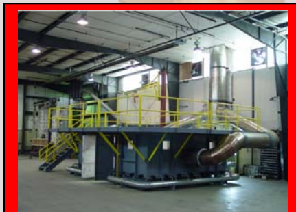
WFCi's New Full Scale Horizontal Furnace.
